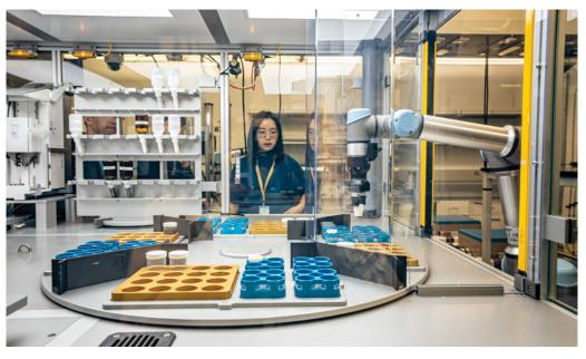
FIGURE 5.6 The A-Lab combines Al-guided synthesis with automated materials characterization
