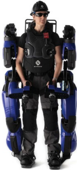
FIGURE 7.6 Sarcos Guardian XO Max wearable exoskeleton
